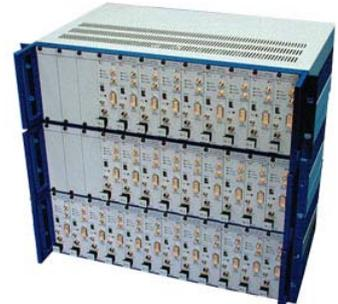
Multi-channel controller consisting of 3 E-500.621 chassis and 30 E-621 modules
