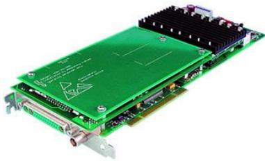
E-761 Three-Axis Digital Piezo Controller Board
