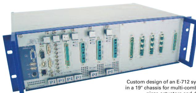
Custom design of an E-712 system in a 19" chassis for multi-combined piezo actuators and drives
