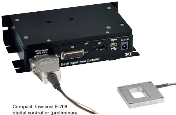
Compact, low-cost E-709 digital controller (preliminary case design) with P-712 piezo-scanner
