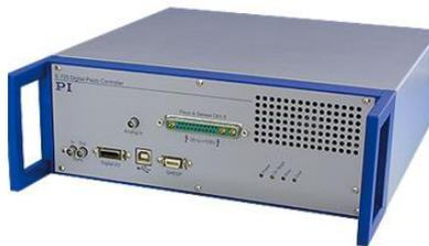
E-725 High-Performance Digital Piezo Controller, 3 Channels
