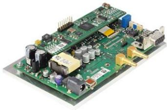
E-609 low-cost digital controller board for OEMs
