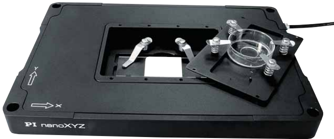
PI nano™ series nanopositioning stages feature a very low profile of 20 mm (0.8), a large aperture for 3 x 1" slides and deliver highly accurate motion with sub-nanometer resolution. Slide / petri dish holders optional
