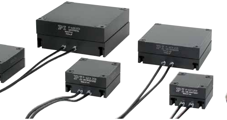
PIHera® XY nanopositioning systems provide travel ranges from 50 x 50 µm to 1800 x 1800 µm
