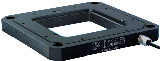
P-541 series nanopositioning Z-stages and Z-tip/tilt stages offer travel ranges of 100 µm with sub-nanometer resolution. They feature a very low profile of 16.5 mm and a large 80 x 80 mm aperture. Versions with strain gauge and capacitive position feedback sensors are available
