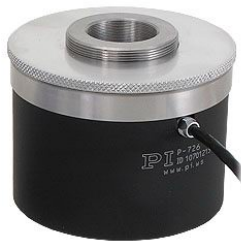
P-726 High-dynamics PIFOC ® objective scanner for heavy, high NA microscope objectives, 100 \mu\text{m} travel range capacitive feedback.
