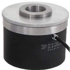
P-726 High-dynamics PIFOC<sup>®</sup> objective scanner for heavy, high NA microscope objectives, 100  $\mu\text{m}$  travel range capacitive feedback.
