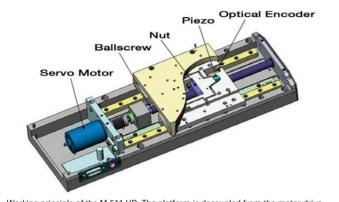
Working principle of the M-511.HD. The platform is decoupled from the motor drive train by the piezo actuator and the flexure guides. This also reduces the inertia of the piezo-driven platform and allows for rapid response
